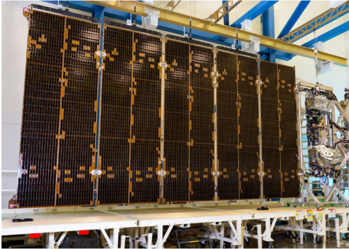
The fully-deployed GOES-R solar array panel. Credit: Lockheed Martin
