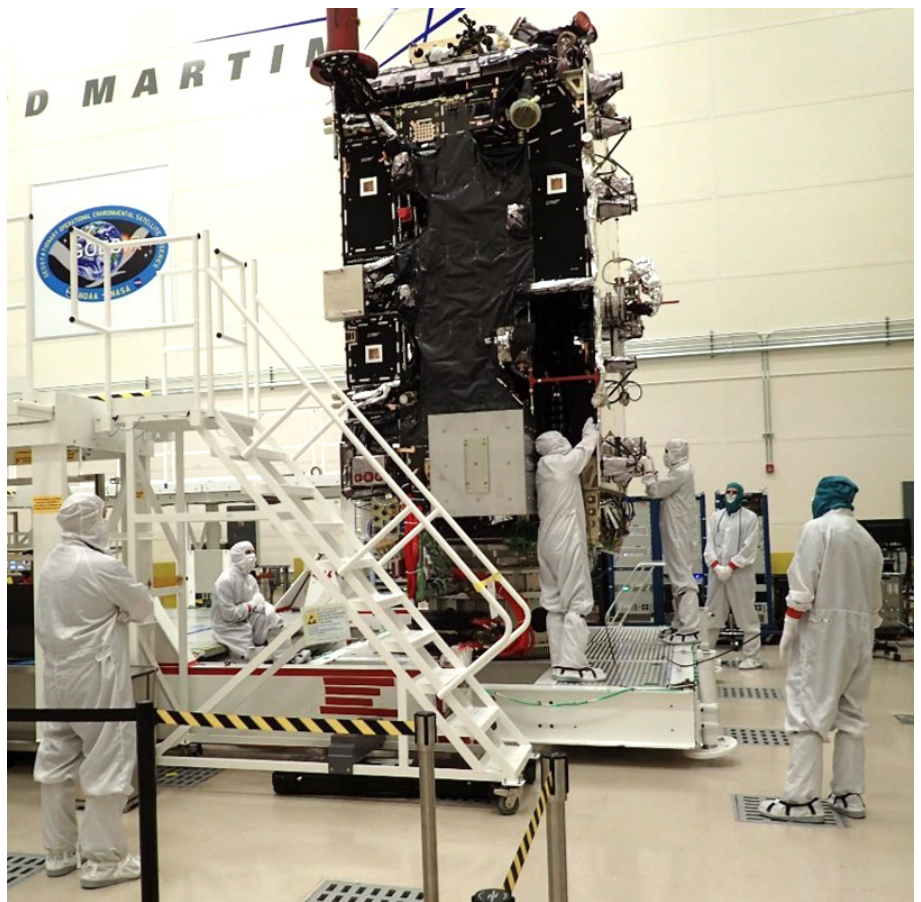
Technicians at Lockheed Martin conduct GOES-T satellite integration activities. Credit: Lockheed Martin
